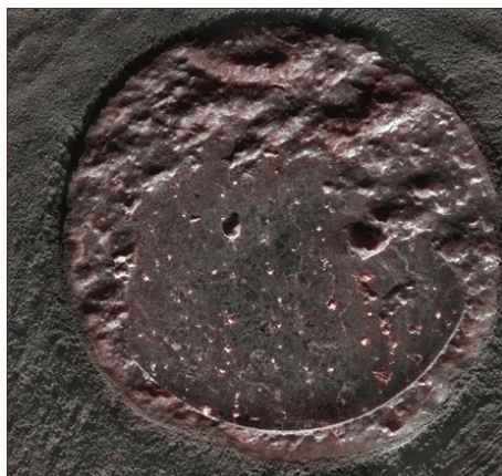
Figure 6-9. A dust free, cleaned and smoothed surface provides a better target for instrument measurements than an “as-is” surface. Abraded/ground surface on the rock Humphrey at the Spirit site. The ground surface shows no obvious artifacts related to the grinding operation, providing a clear view of the textural details of the rock and a work surface suitable for interrogation by compositional instruments. Brushed and abraded circle is 45 mm diameter. Grayscale image from the MI camera, merged with color from Pancam imager. Credit to JPL/NASA/MSSS.
